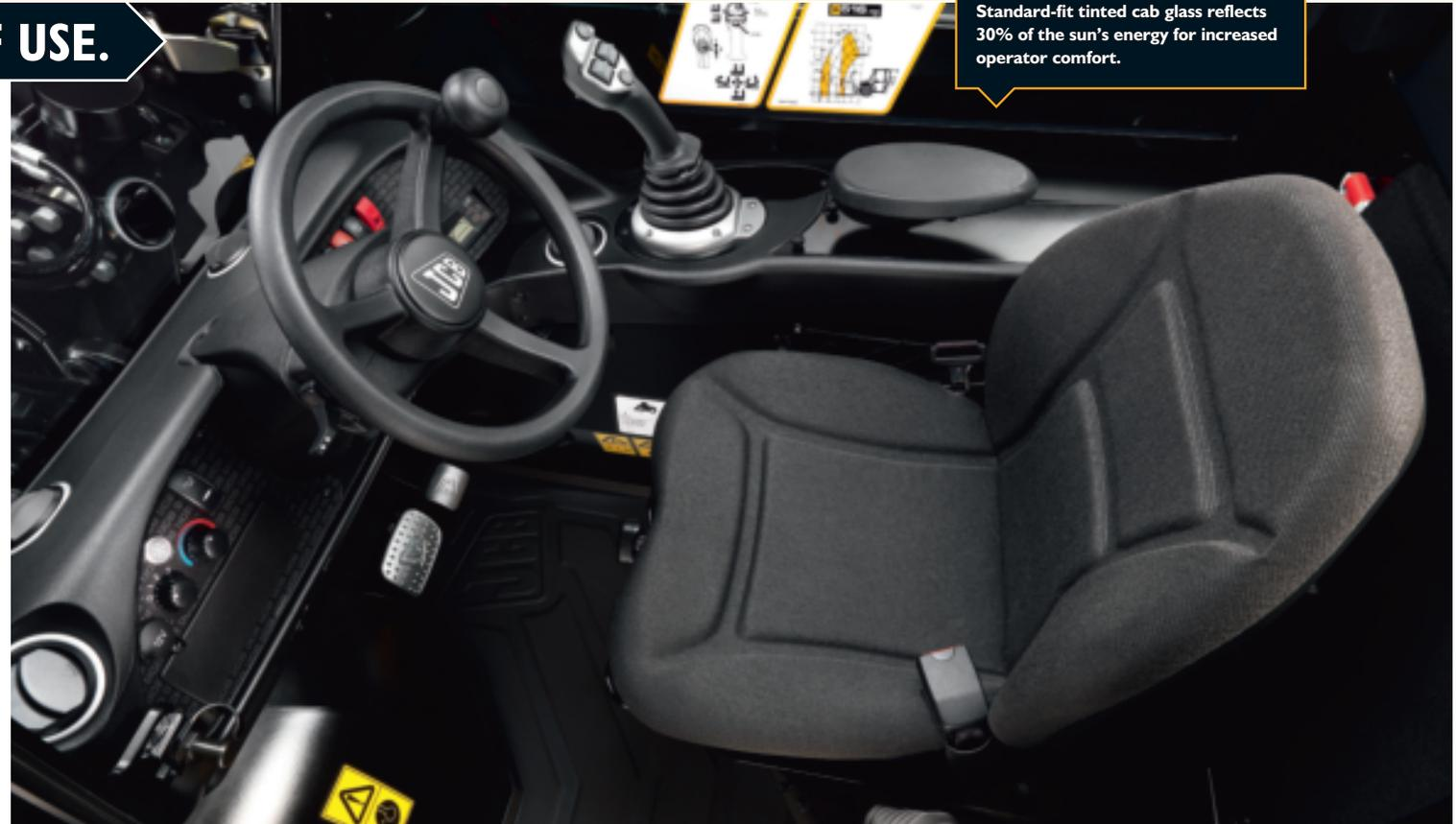
Standard-fit tinted cab glass reflects 30% of the sun's energy for increased operator comfort.
