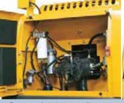
• Easy access for hydraulic pump filters.
